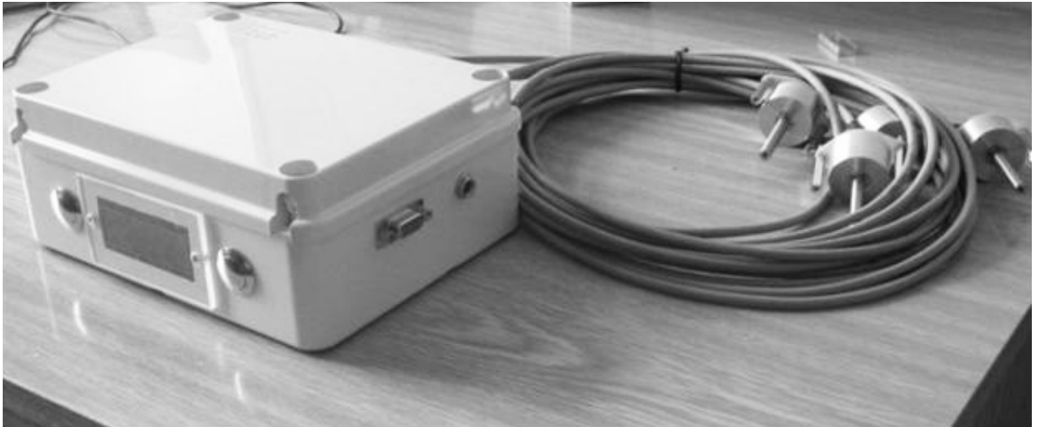
Fig. 4. The microcontroller unit controlling magnetic transducers data transfer to the host computer. The transducers in the final performance are in the right part of the picture.
