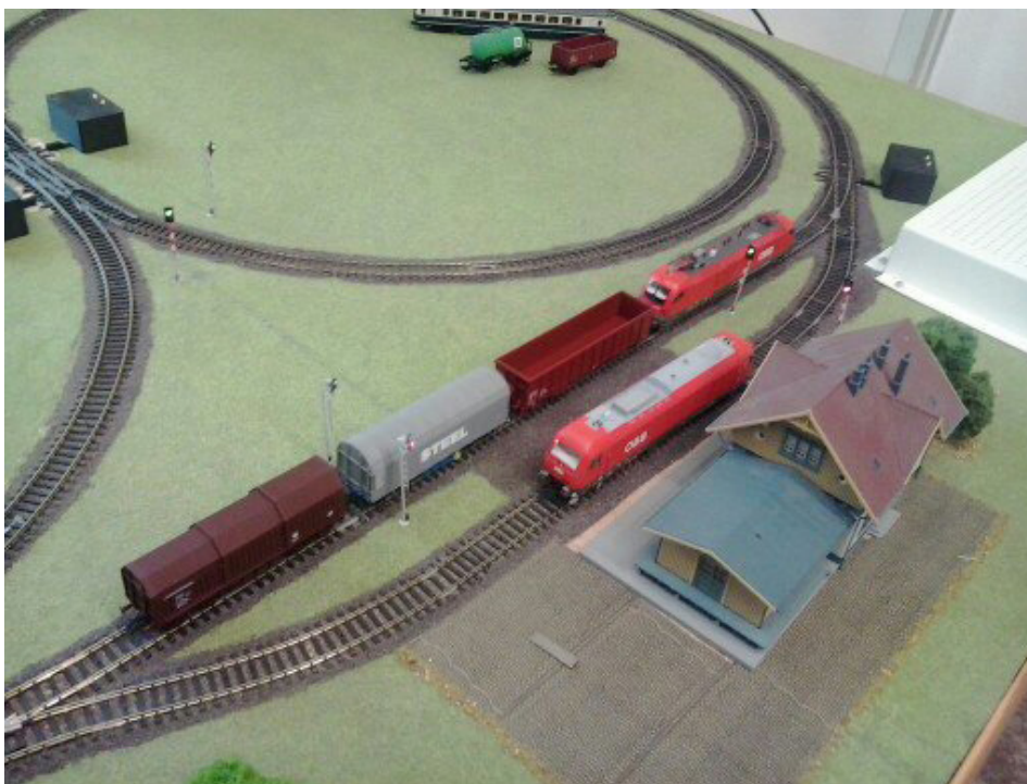
Figure 5: Digital control enables to control more locomotives that are specified by unique id.
